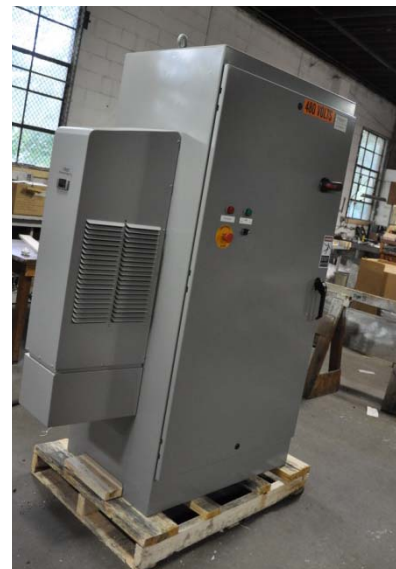
Below: 480V 350A 3 Phase transformer primary driver. System has remote power monitoring transducers, as well remote command and control signals to and from a PLC. System used outdoors, NEMA 4 w/ Air Conditioning unit. Petrochemical application.
