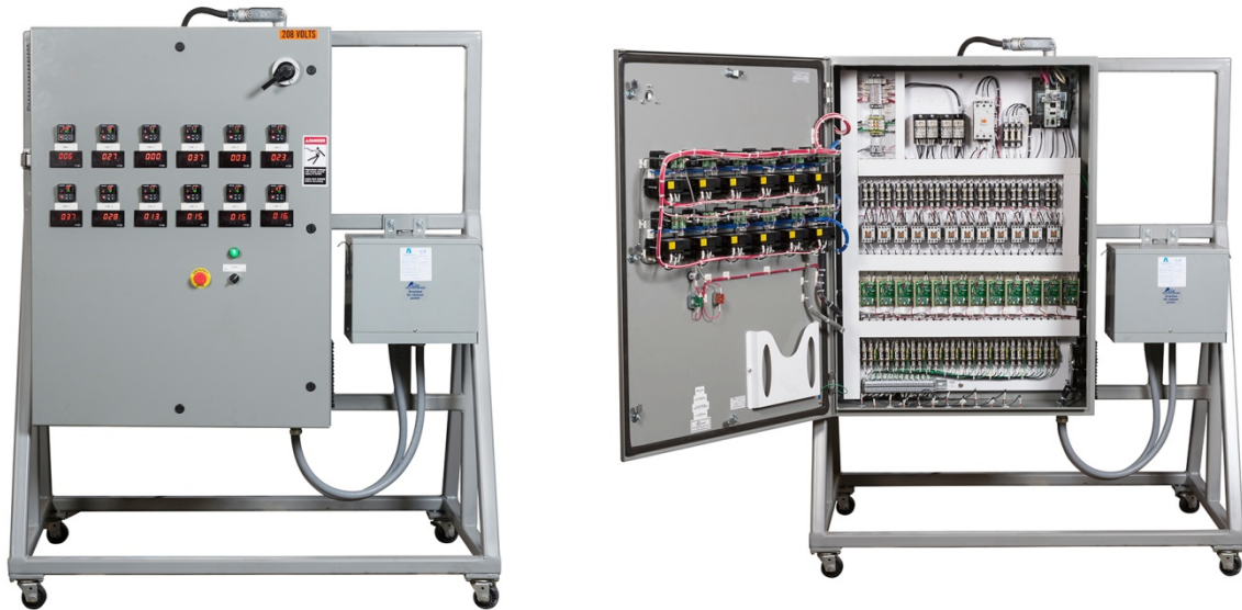
Above: 12 Zone system for use at NASA. Each zone has PID control, computer communications and voltage output monitoring. A custom frame was built so system could be mobile. Custom step down transformer was installed.
