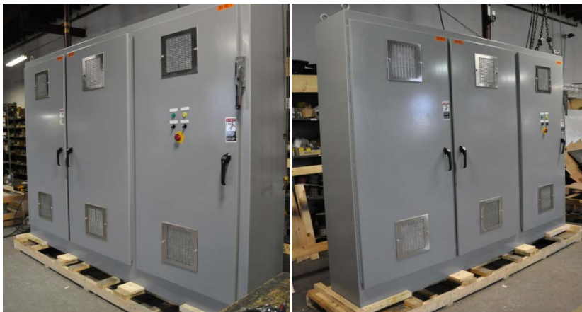
Below: 480V 350A 3 Phase transformer primary driver. System has remote power monitoring transducers, as well remote command and control signals to and from a PLC. System used outdoors, NEMA 4 w/ Air Conditioning unit. Petrochemical application.
