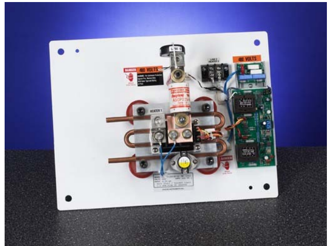
Single phase 480V 250A water cooled SCR also with current limit and soft start option.
