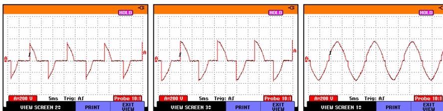
25% output or 60V RMS.    50% output 120V RMS.    99.5% output or 238.8V RMS
